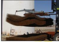
The Mesh Handler is designed primarily for use with a forklift; however pick-up points have been provided for use with a crane. The user must determine the proper safety procedures and requirements when using the Mesh Handler with a crane.
