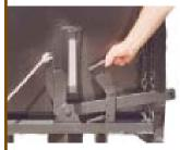
prevents accidental discharge when transporting a load. Must be disengaged before hopper will dump.
