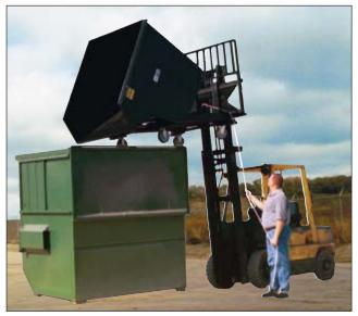
**Universal Fit** - Can be used with both straight-mast and extendable-reach forklifts. Pocket Base accommodates forks up to 10" wide and 2½" thick.
