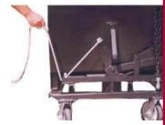
can be used to trip the hopper from the ground or from the operators seat.
