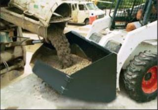
Extra High Back helps keep "concrete splatter" off the loader
