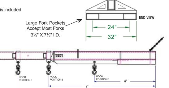
CAUTION: BE AWARE THAT FORKLIFT RATED CAPACITIES <u>DIMINISH RAPIDLY</u> WHEN THE LOAD CENTER IS MOVED OUT. WHEN USING THE JIB, MAKE SURE YOUR FORKLIFT HAS ADEQUATE CAPACITY TO HANDLE THE DESIRED EXTENDED LOAD. SEE BOTH THE HEAVY DUTY JIB AND YOUR FORKLIFT OPERATOR'S MANUALS FOR MORE INFORMATION. LOAD CAPACITIES SHOWN HERE ARE FOR THE JIB ITSELF AND DO NOT IN ANY WAY REFLECT THE LIFT CAPACITY OF THE FORKLIFT.
